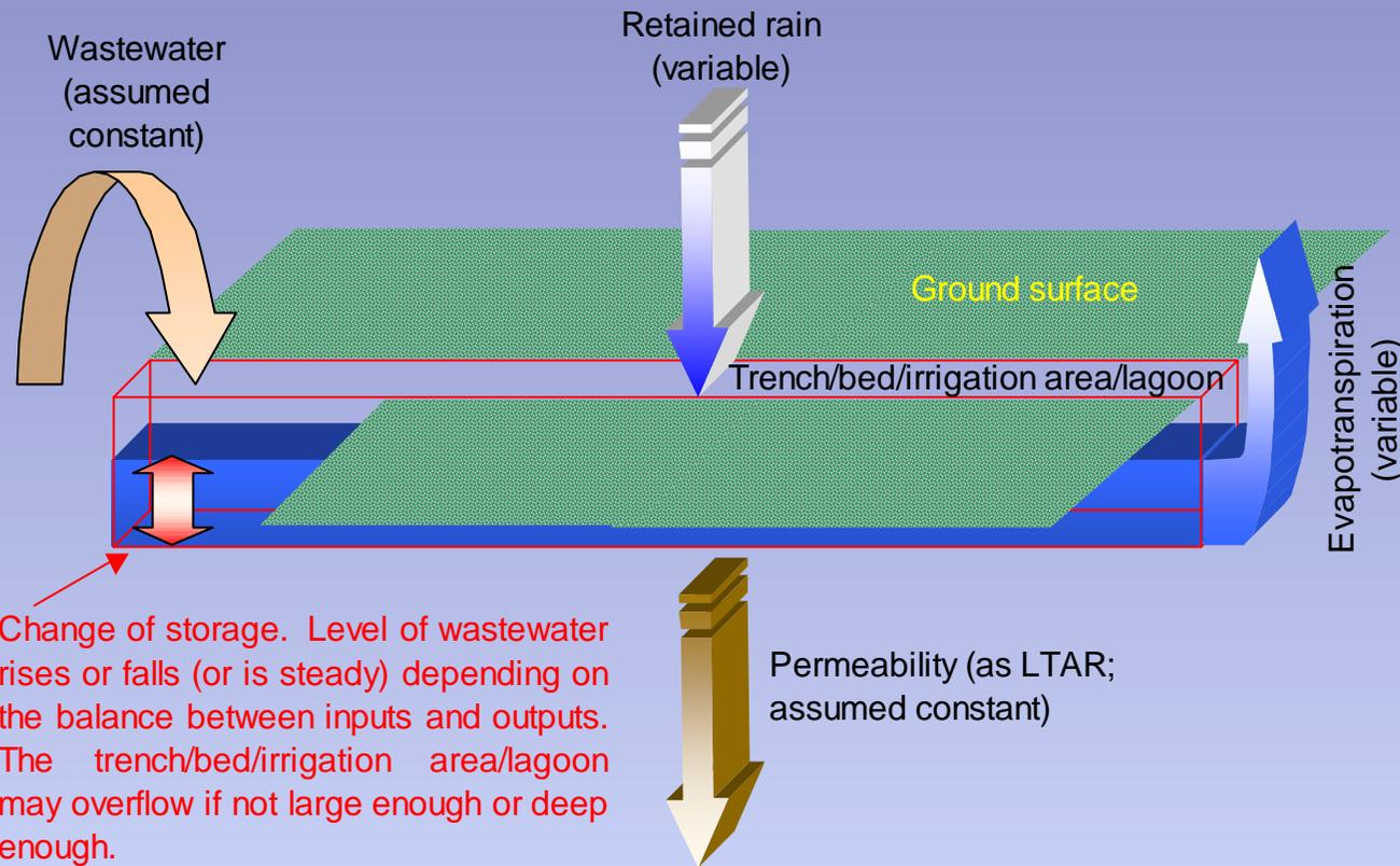
Change of storage. Level of wastewater rises or falls (or is steady) depending on the balance between inputs and outputs. The trench/bed/irrigation area/lagoon may overflow if not large enough or deep enough.
