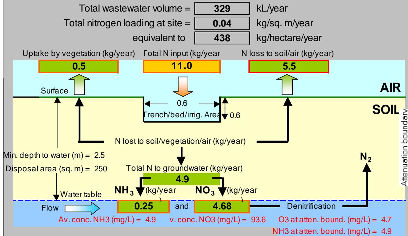
Aver. conc. in g'water is calculated to a depth of 1 m below water table
