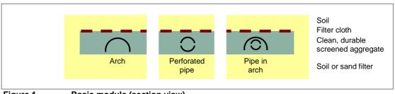
Figure 1 Basic module (section view)
