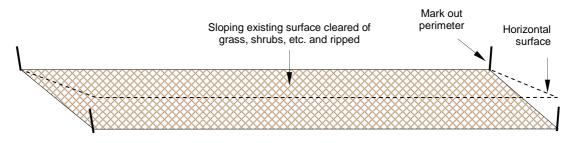
Figure 10. Steps 1 – 5. Protect, clear, mark out, add gypsum if required
