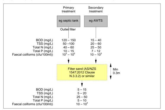
Figure 7. Approximate treatment efficiencies of filter sand
