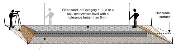
Nominally 1:3 outer batter if no retaining wall. Repeat at both ends of system, or grade to natural surface.
