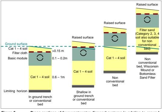
Figure 5. Cross sections of four wastewater disposal systems in relation to ground surface and the depth to a limiting horizon. Adapted from Converse and Tyler (2000) and Cromer (2004)
