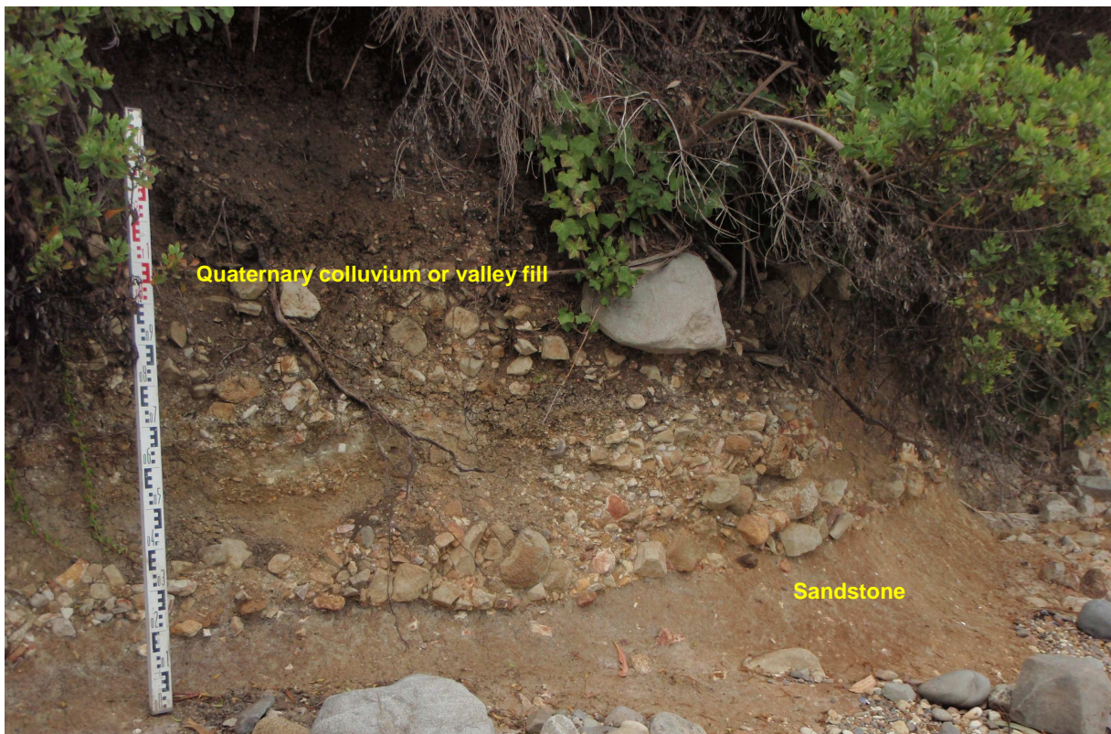
Plate 12 (above). Detail of the base of the coastal escarpment up to 15m high in front of (address). The staff is 1.3m high. Quaternary colluvium or valley fill overlies conglomerate and sandstone.
