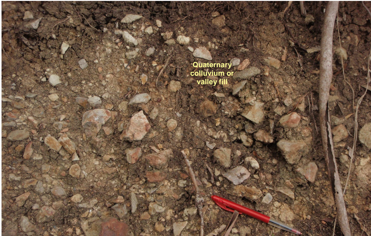
Plate 6 (above). Detail of the weakly consolidated material interpreted as Quaternary colluvium or valley fill, exposed on the (deleted). The material is a near-clast supported conglomerate of 50% angular Permian sandstone and siltstone clasts to 0.1m, and subrounded dolerite clasts to 0.2m, in a moderate plasticity gravelly clay. The proportion of sedimentary to dolerite clasts is about 3:1. Shown here is mostly the former.
