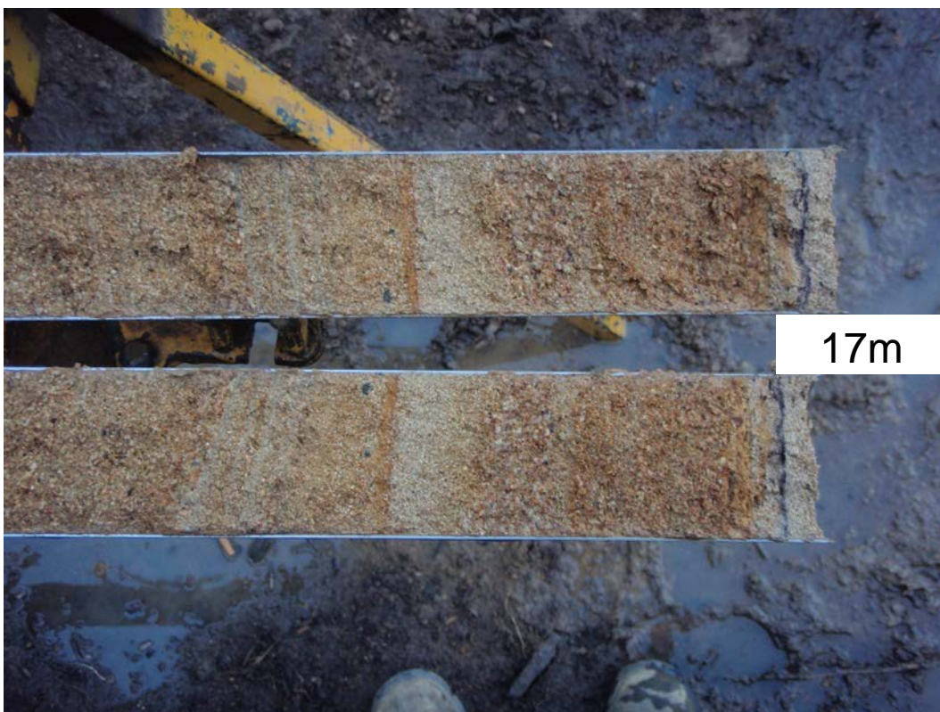
Weakly cemented low strength and coarse grained sandstone in DDH C near 17m.
