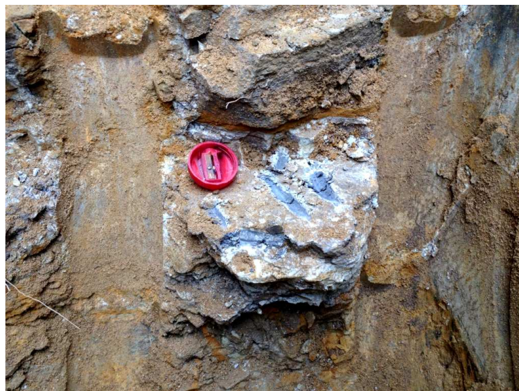
Plate 21 (below). Detail of the end of Trench B, showing grey-blue, high plasticity clay coatings several millimetres thick on a dipping joint surface. Slipping on these coatings is a likely mode of localised failure for the colluvial cover.
