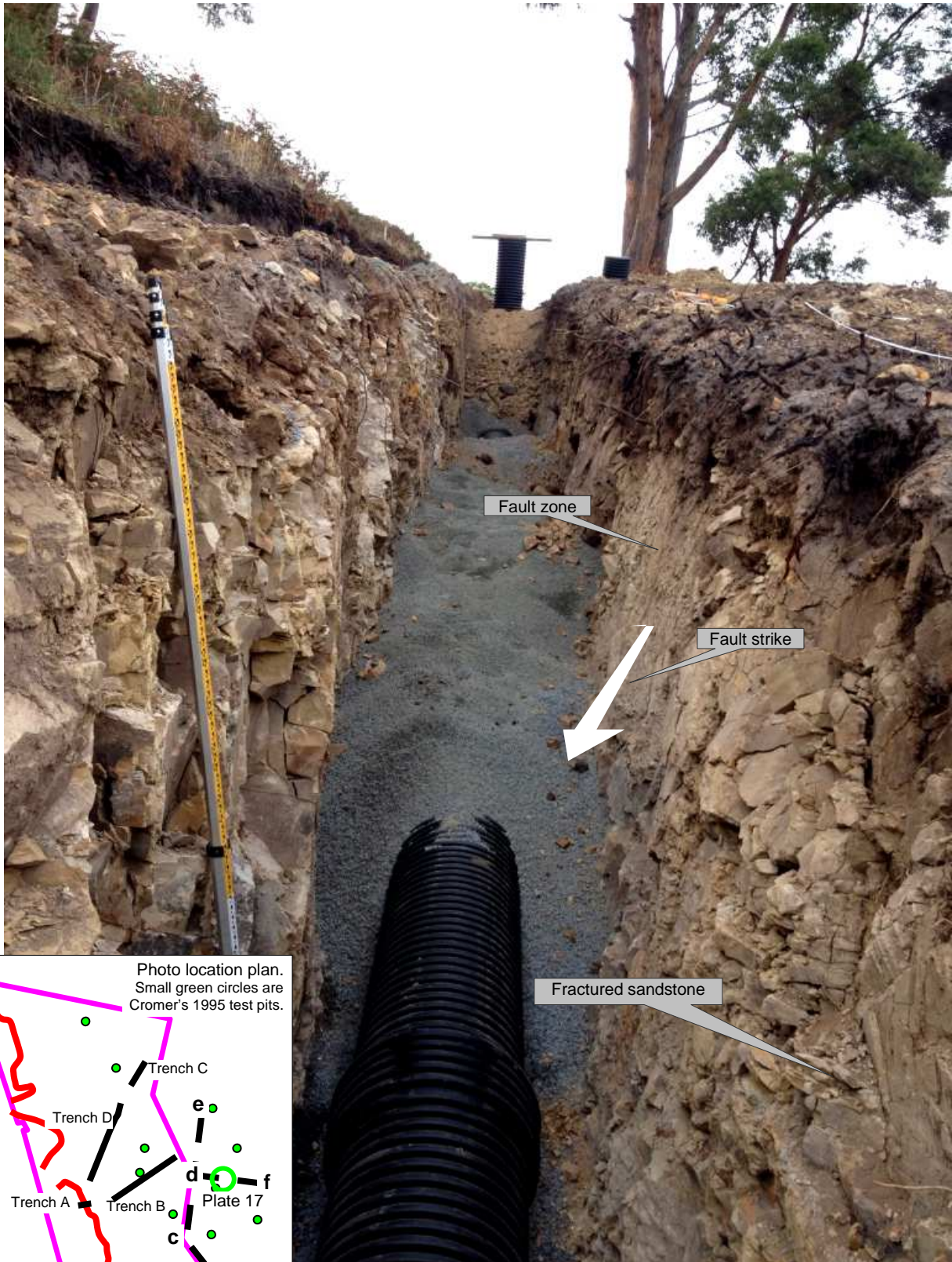
Plate 17. Service trench abcdef between d and f, looking upslope towards f. The fractured sandstone exposed in the services trench at this location appears to be in-situ. A narrow fault zone about 0.5m wide crosses the trench at an oblique angle (arrowed).
