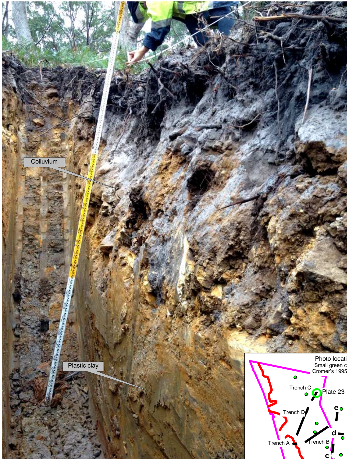
Plate 23. View north northwest at the higher end of Trench C, 17.5m long. This excavation up to 2.6m deep exposed colluvial materials over high plasticity clay, with no bedrock.
