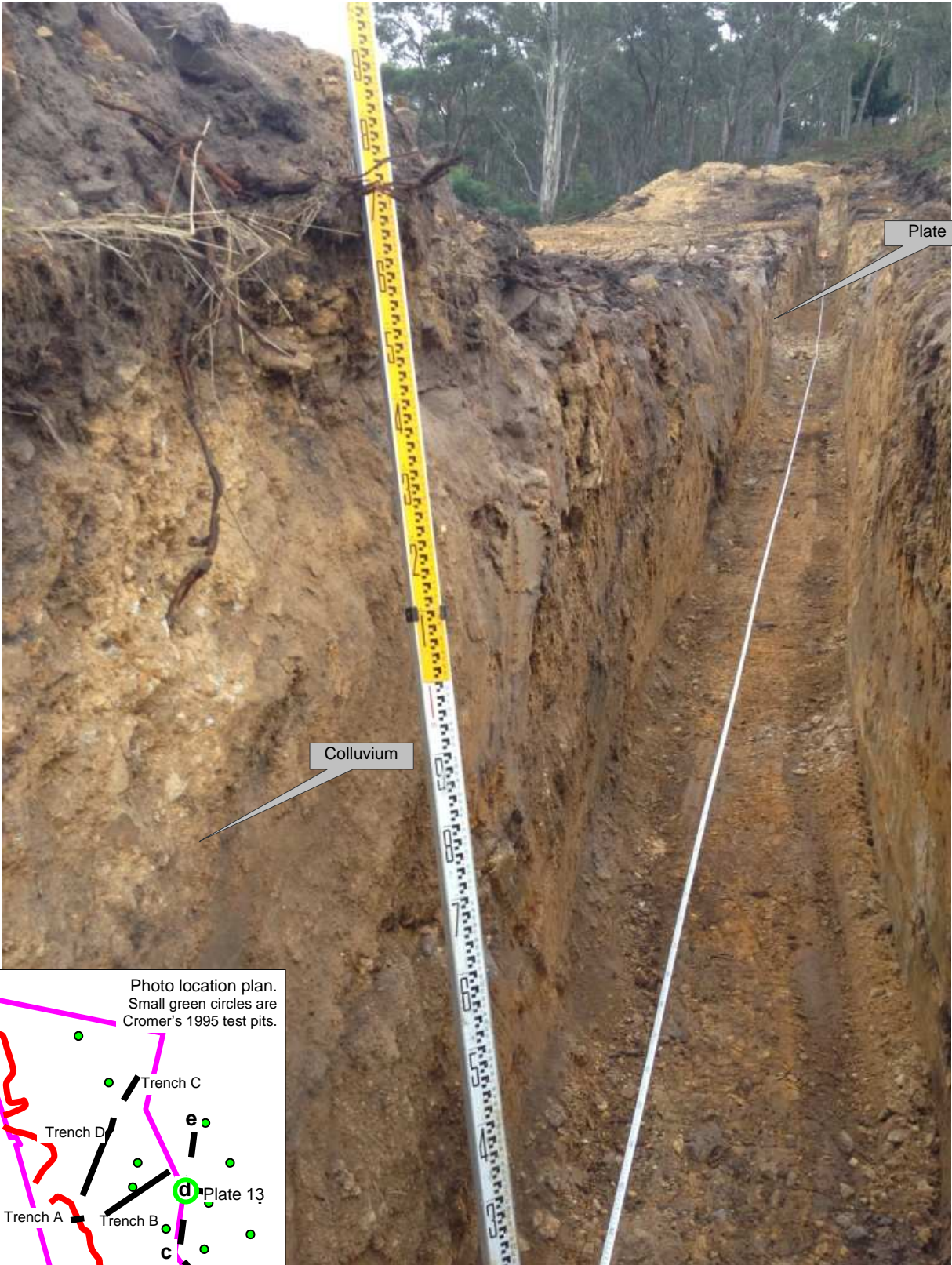
Plate 13. Service trench abcdef at d, looking upslope to e. The profile is mainly dry non-plastic colluvium, interspersed with patches of strongly fractured sandstone which may be in-situ bedrock, and other patches of strongly fractured sandstone underlain by colluvial material and therefore not in-situ.
