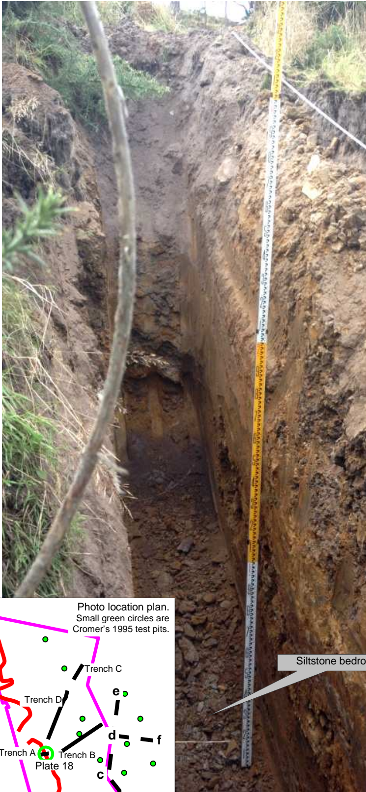
Plate 18. Investigation trench A, about 8m long, was dug across the headscarp of landslide #874. The failure surface was probably close to the camera, but not apparent. Colluvium overlies highly weathered siltstone bedrock, exposed in the base of the trench, and dipping 11^{\circ} to 260^{\circ} T.
